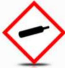
Compressed Gas Hazard
